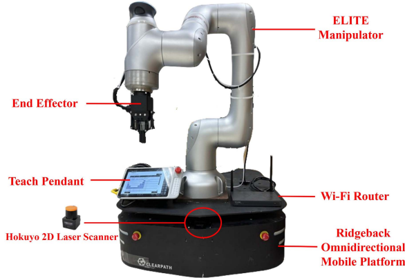
Fig. 7. Hardware Configuration of the Mobile Manipulator.
