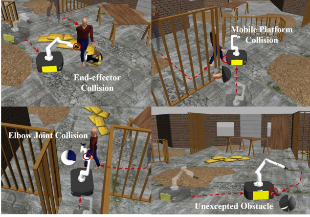
Fig. 5. Gazebo Simulation Scenarios. The four simulation scenarios cover collisions with the end-effector, elbow joint, mobile base, and an unexpected obstacle to ensure comprehensive validation.
